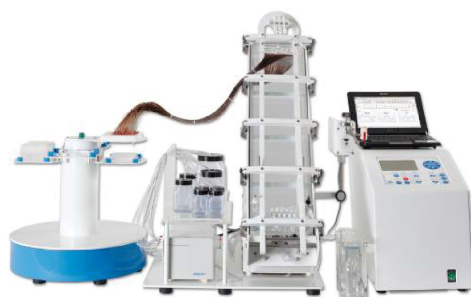
Figure 1. Free-Flow Electrophoresis Free-Flow Electrophoresis was performed at FFE Service in Feldkirchen (Germany). Analytes are separated based on their charge in a flow chamber (left). The separated analytes are directly collected in 96-well plate format, which enables semi-preparative purification of analytes.
